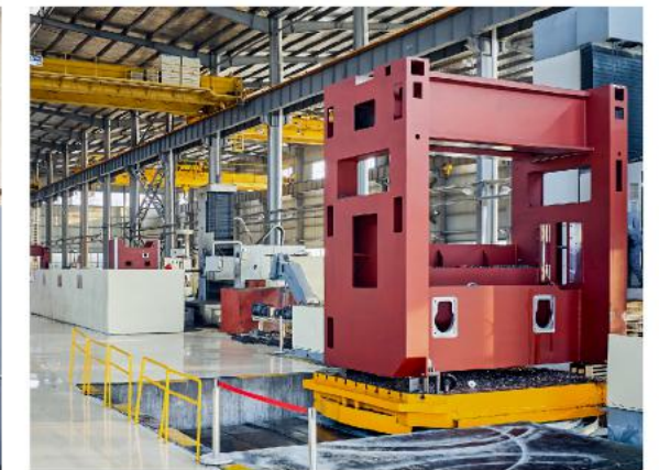
FBC160r数控滑枕剖台式铣镗床 FBC160r CNC sliding table horizontal milling and boring machine
