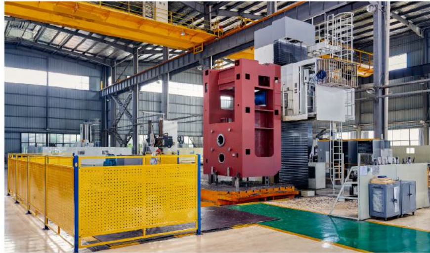
FBC160r数控滑枕剖台式铣镗床 FBC160r CNC horizontal ram milling and boring machine
