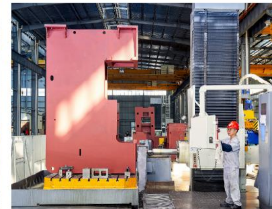
TK6516A数控刨台式卧式镗铣床 TK6516A CNC planer table horizontal boring and milling machine
